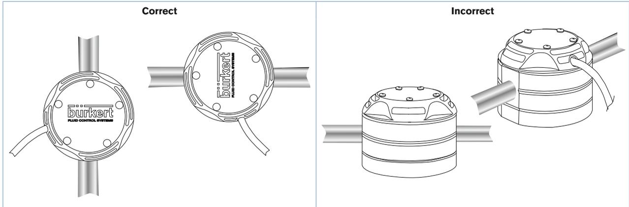
The pipe must be filled with liquid and free from air bubbles. Avoid air purge of the system which would cause damages and to prevent damage from dirt or foreign matter, we strongly recommend the installation of a 250 µm strainer as close as possible to the inlet side of the meter.
